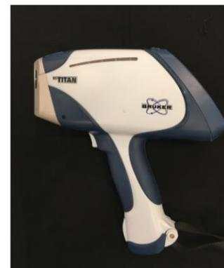
Appareil XRF portable
